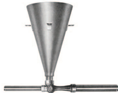
Fig. 19. FIG. 267 HOPPER-EQUIPPED EDUCTOR. This economical unit is available from stock with body and nozzle in cast iron, bronze, 316 stainless steel, Kynar and PVC. Hoppers are stocked in Type 304 stainless steel (1, 1 1/2 & 2" sizes) and are also available in galvanized steel, brass, aluminum and PVC.
