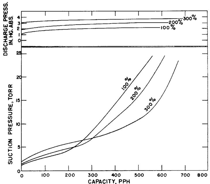
Fig. 7 Typical effect of steam rates on stage performance
