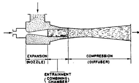
Fig. 1 Fundamental steam jet-vacuum pump parts
