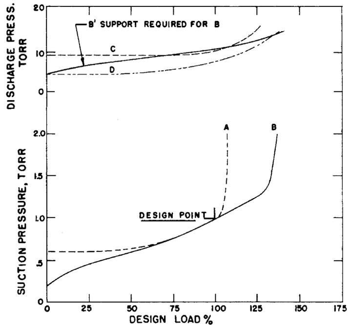
Fig. 10 Typical combination of two noncondensing stages
