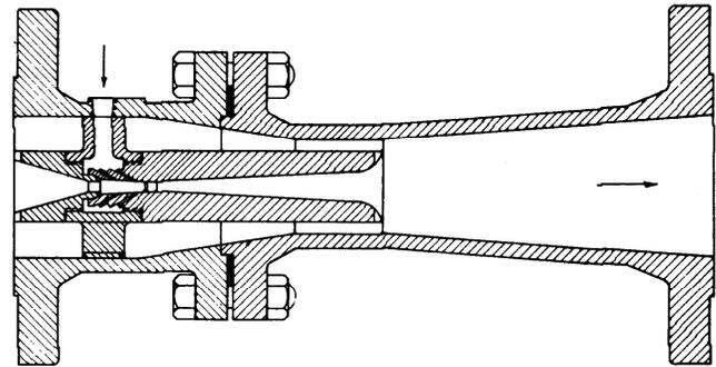
Fig. 1 Venturi desuperheater
