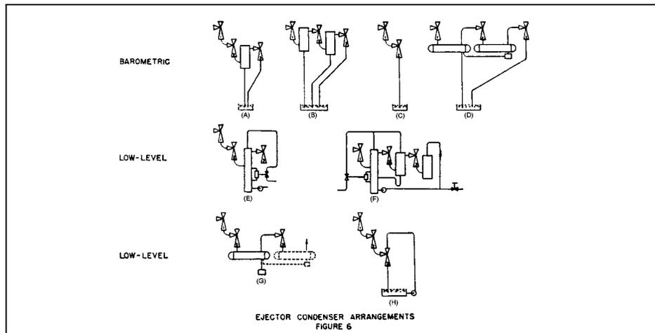
Figure 3. The type of inter-stage cooler-condenser used may be varied with the application requirements.
