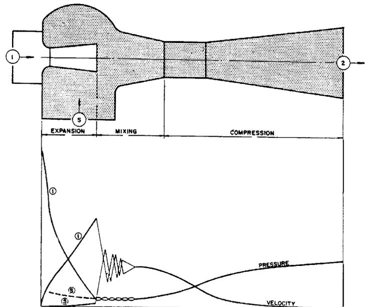
Figure 2. A plot of the ejector process.
