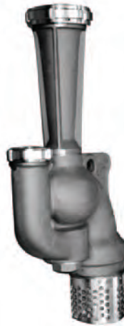
Fig. 24. FIG. 222 PORTABLE EDUCTOR. Is designed for use as an auxiliary with a pump where the suction lift is too great for the pump alone. Made of anodized aluminum, bronze or other materials as required.
